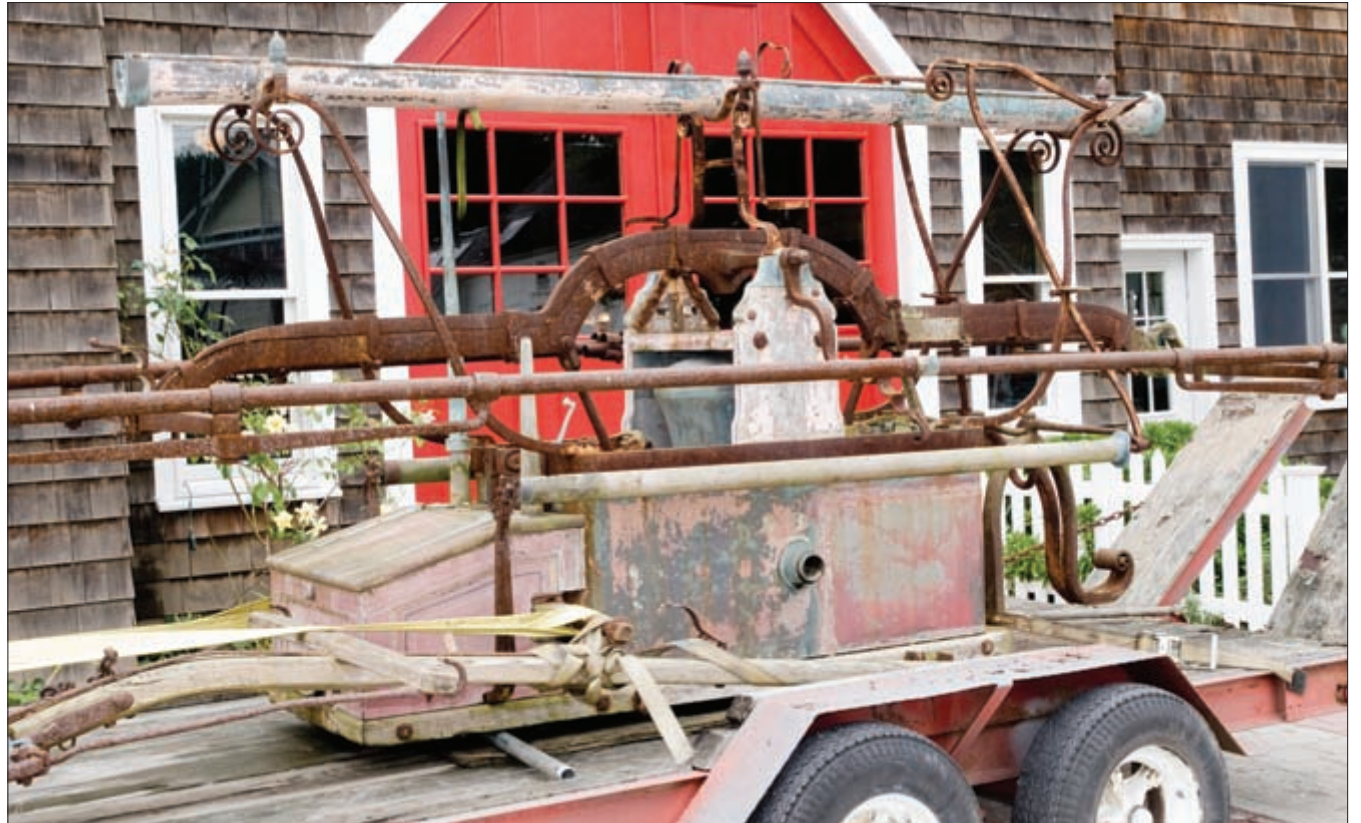
The Jamestown Fire Department Memorial Museum recently acquired a pre-civil war "hand tub" from the South County Museum. Built by Hunneman & Co. in Roxbury, Mass., the antique fire engine is slated for restoration to working condition.
